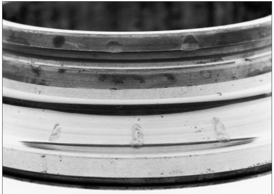
57: False brinelling on the ball bearing
