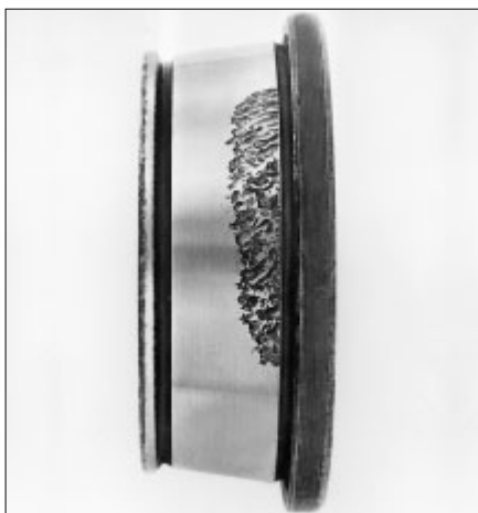
40: Tilted track on a tapered roller bearing
