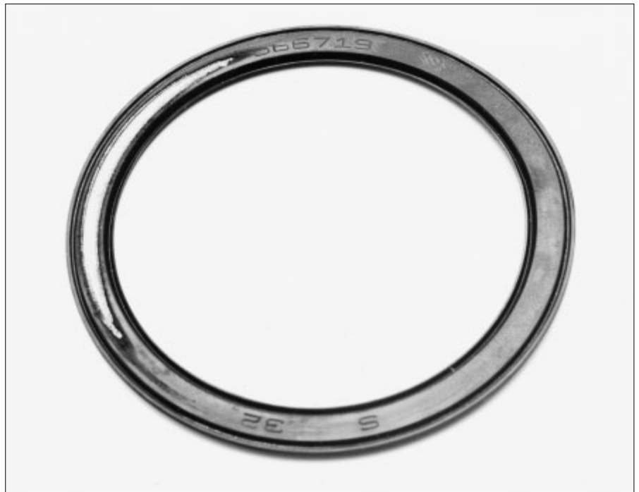
22: Seal damage due to lateral grazing
