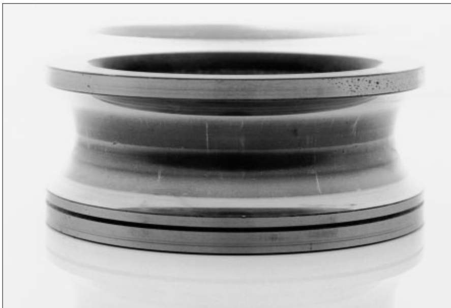
28: Track with surface wear
