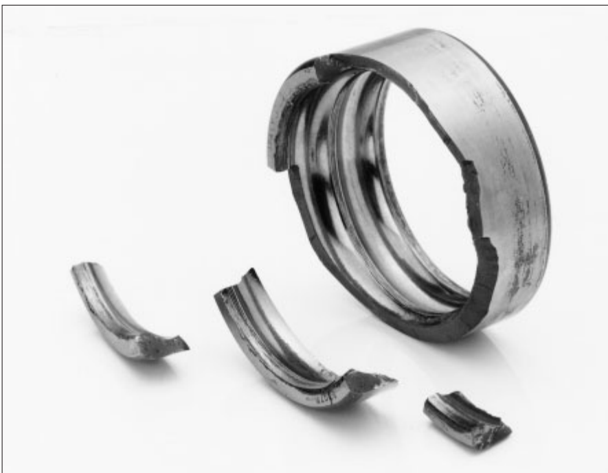
65: Crack in outer ring in circumferential direction
