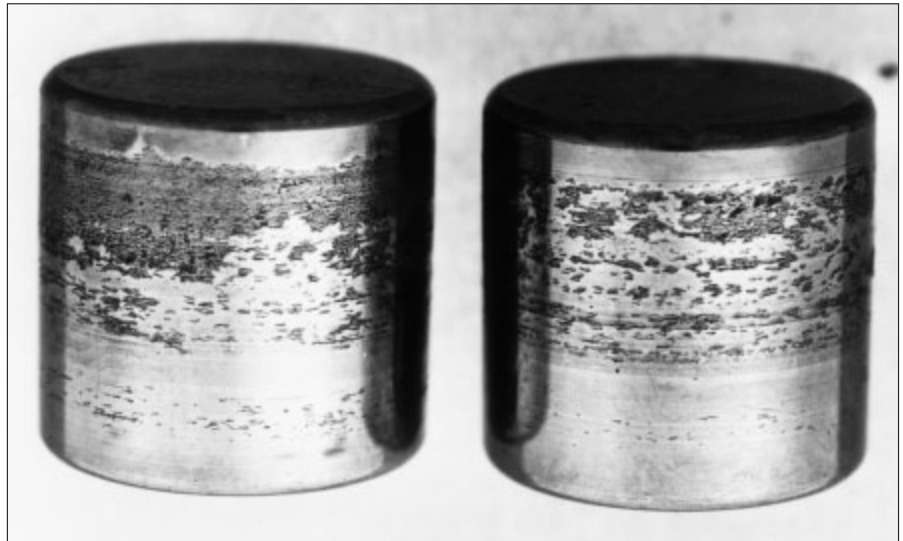
74: Slippage tracks on cylindrical rollers
