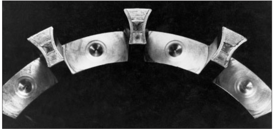
92: Fractured cage-rivet connections may result from vibration stress.
