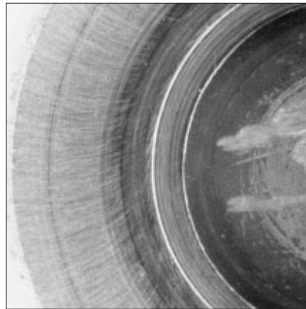
83: Cross profile chart of a worn tapered roller face
