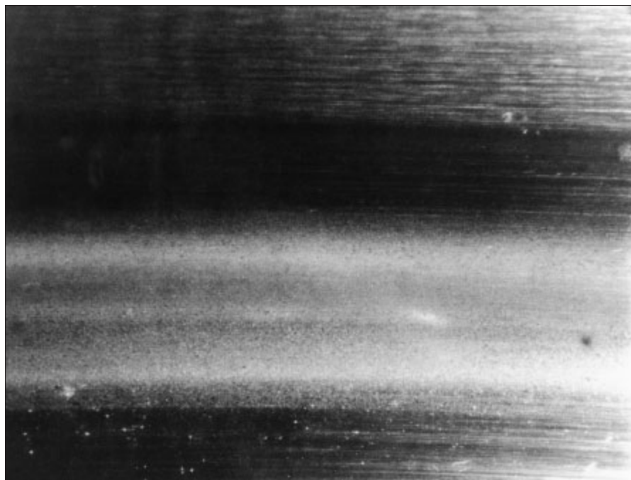
66: Worn, roughened raceway
