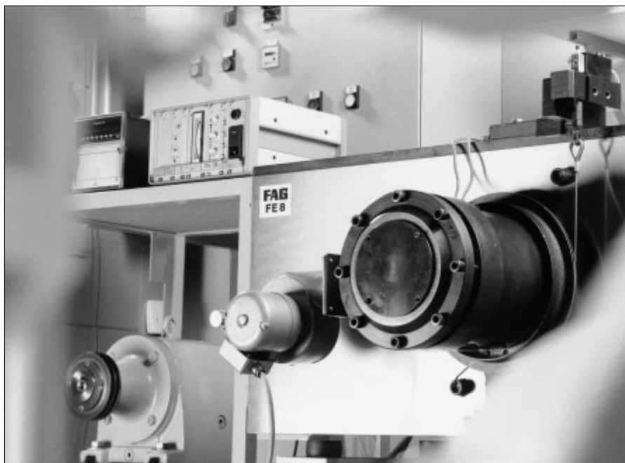
107: Test rig for determining lubricant quality
