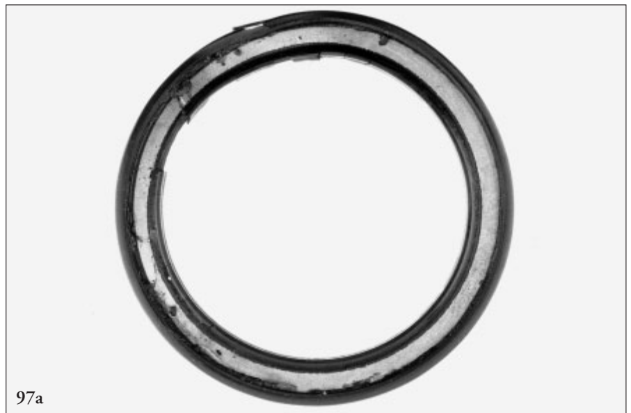
97: a: Hardened sealing with wear and fractures
