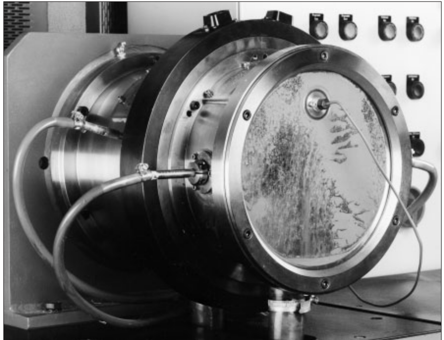
114: Test rig for inspecting the efficiency of rolling bearing seals
