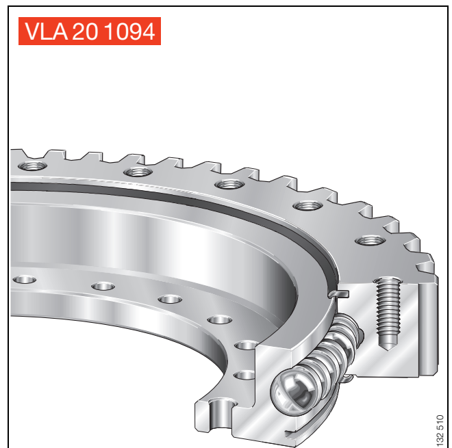
Figure 1 · Designation – example of four point contact bearing
